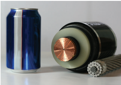
A solid dielectric underground cable is significantly larger than a standard conductor that hangs from an overhead structure. The CapX2020 345 kV overhead structures will carry at least six conductors.
